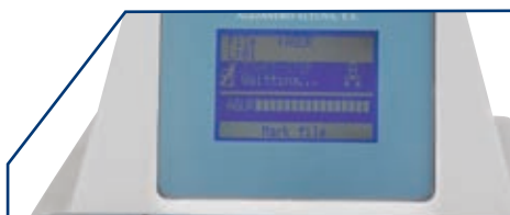
1 Pantalla LCD 55mm x 38 mm.
